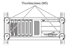
**10** Install the second enclosure to the rack in the same way.
